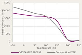
Figure 4 - Tensile Modulus between -50°C and 250°C
