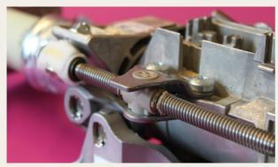
Figure 1 - Steering column adjustment assembly
